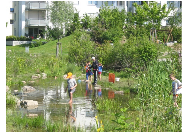
Shallow slopes, low water depth and stable edges minimise the need for fences and illustrate a designed approach to health and safety
